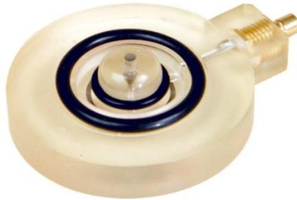
Figure 3. The epoxy resin disk complete with the center cathode and ring anode. The O-rings are placed for demonstration, but the required PTFE membrane and paper spacer are omitted. (Hansatech, n.d.)
