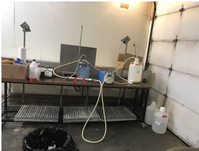
Figure 2-4. Filtering apparatus used to concentrate Diluted and Clarified Egg Yolks into Hollow Fiber Concentrated Antibody.
