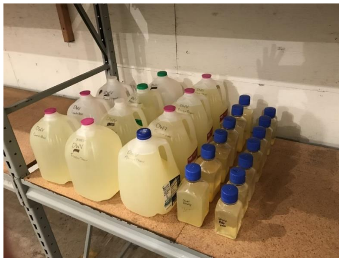
Figure 2-3. Diluted and Clarified Egg Yolks after lipid layer is discarded. Note the off-yellow, cloudy color.
