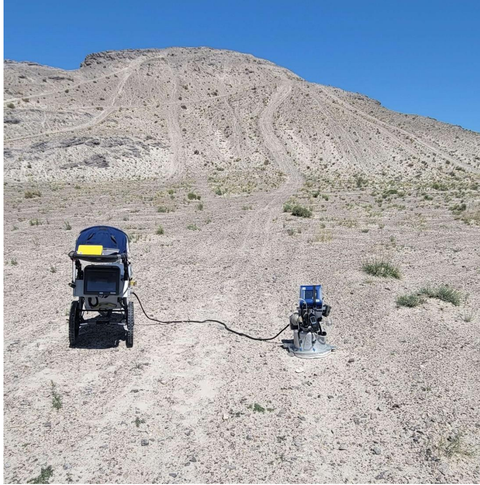
Figure 4: Photograph of the PI-SWRL (right) with computer, battery and control box mounted on carriage (left).
